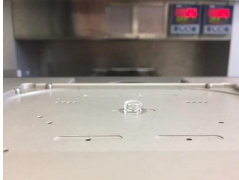
Fig. 1. Bioprinted 3D vascular structure using collagen-hyaluronic acid hydrogel and progenitor cells
